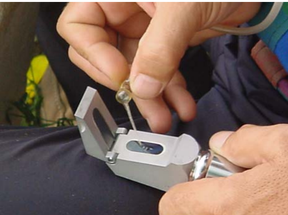
Figure 3. Determination of sugar concentration using a refractometer
