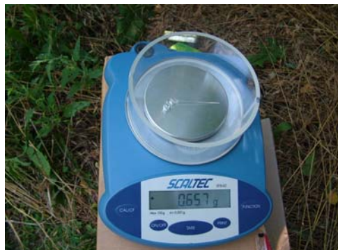
Figure 1. Weighting the capillaries used for nectar extraction
