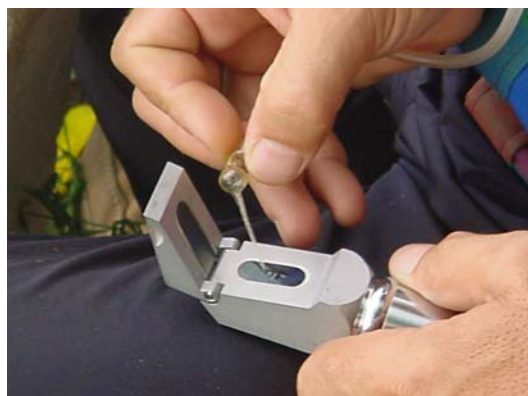
Figure 3. Determination of sugar nectar concentration using a refractometer
